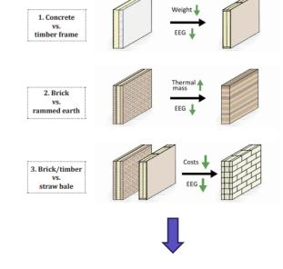
27-77% reduction compared to concrete, masonry and steel
